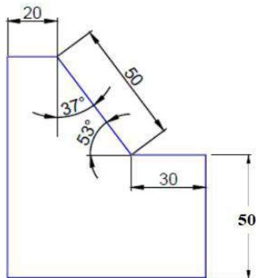
2. Draw the following arrow mark by using any CAD software, and add complete dimensions. Also list the commands used in sequence.
